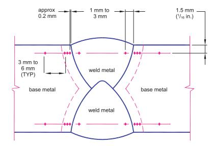
NOTE HV10 measurement for HAZ requires 0.04 in. (1 mm) minimum spacing between indentations. In some cases, it is acceptable that hardness measurement location is off the line in order to satisfy the minimum spacing requirements.
