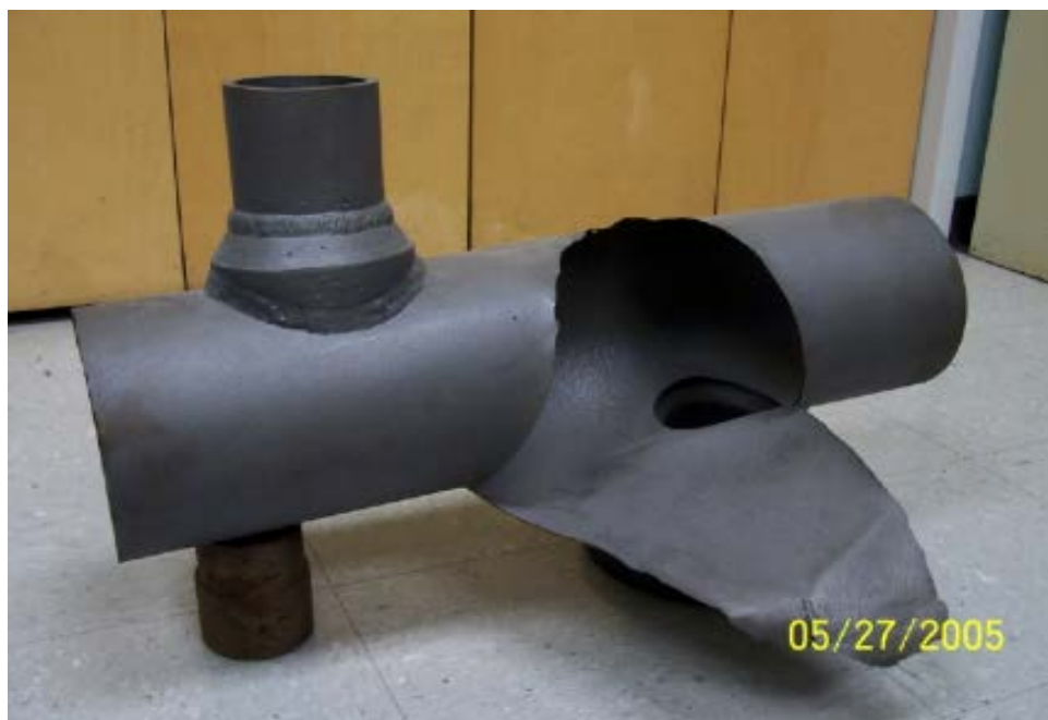
Figure 1—NPS 8 Carbon Steel Piping Failed Due to Sulfidation Corrosion ( H_2 Free)
